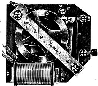
If it is desired to ascertain and correct the fault, open the back and lift the backstop lever G, which will hold the driving click E out of engagement with the wheel A, and spin the wheel A to find undue friction. If the wheel and hands revolve quite freely, there is only one thing more to look at, viz.: the flat steel spring F, which must be just strong enough to propel the hands, but not too strong for the electro-magnet B to pull it over. It may be easily adjusted by the capstan screw.
